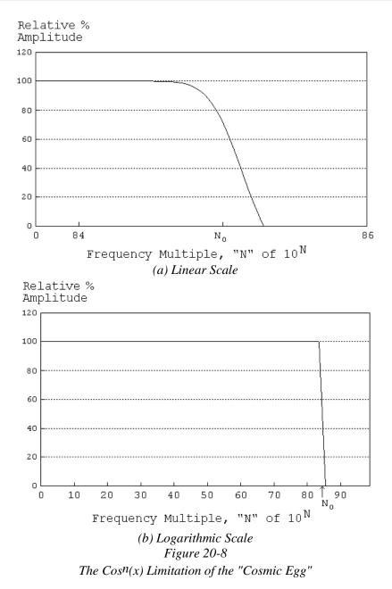
The cutting-off depicted in Figure 20-8, above can be calculated as follows. At the top of Figure 20-9, on the following page, the relative amplitude curve of Figure 20-8(a) is re-depicted. Immediately below it the slope, that is the rate of change, of that curve is depicted. Beneath that slope depiction is depicted the slope of that slope. And beneath that is depicted its slope.
