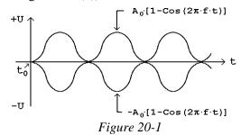
Reexamination of this wave form reveals two problems. One, that it is an immediate mutual annihilation, will be dealt with shortly below. Of concern now is that an infinite rate of change still remains; the envelope of the oscillation has an infinite rate of change at  $t=t_0$  as can be seen in Figure 20-2, below, which displays the envelope.
