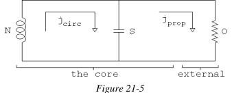
Equivalent Model of the Core
